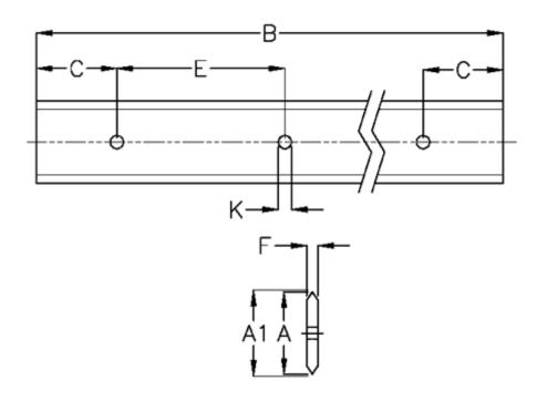
$\begin{array}{lll} A & = 76 \\ A1 & = 76.81 \\ B & = 1616 \\ C & = 43.0 \\ E & = 90 \\ F & = 9.12 \\ For bearing = J54 \end{array}$
